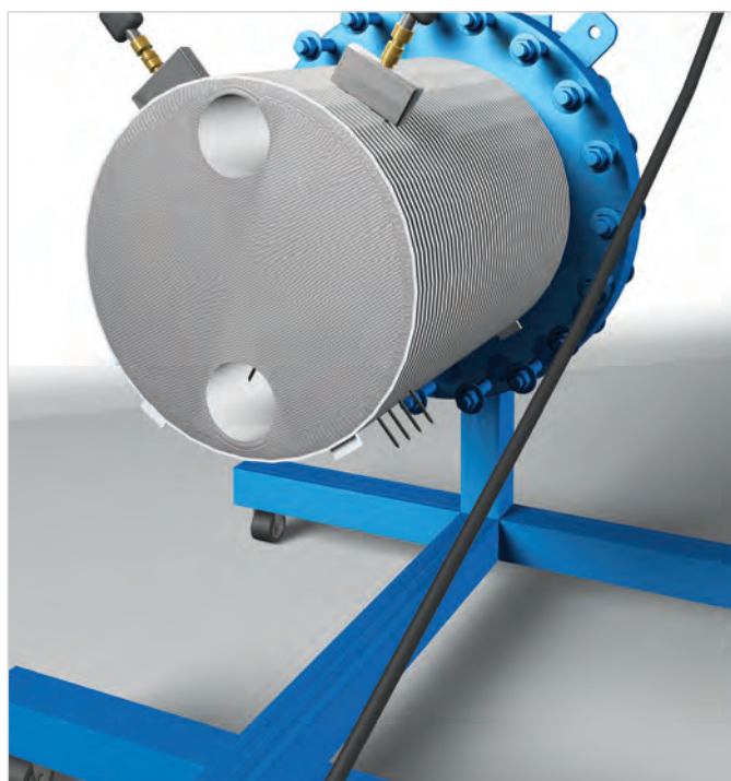
A special Pressure Cleaning Wand Accessory enables cleaning of shell-side channels in the plate pack with the core removed.
