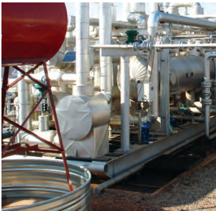
Compact, skid-mounted propane condenser.
